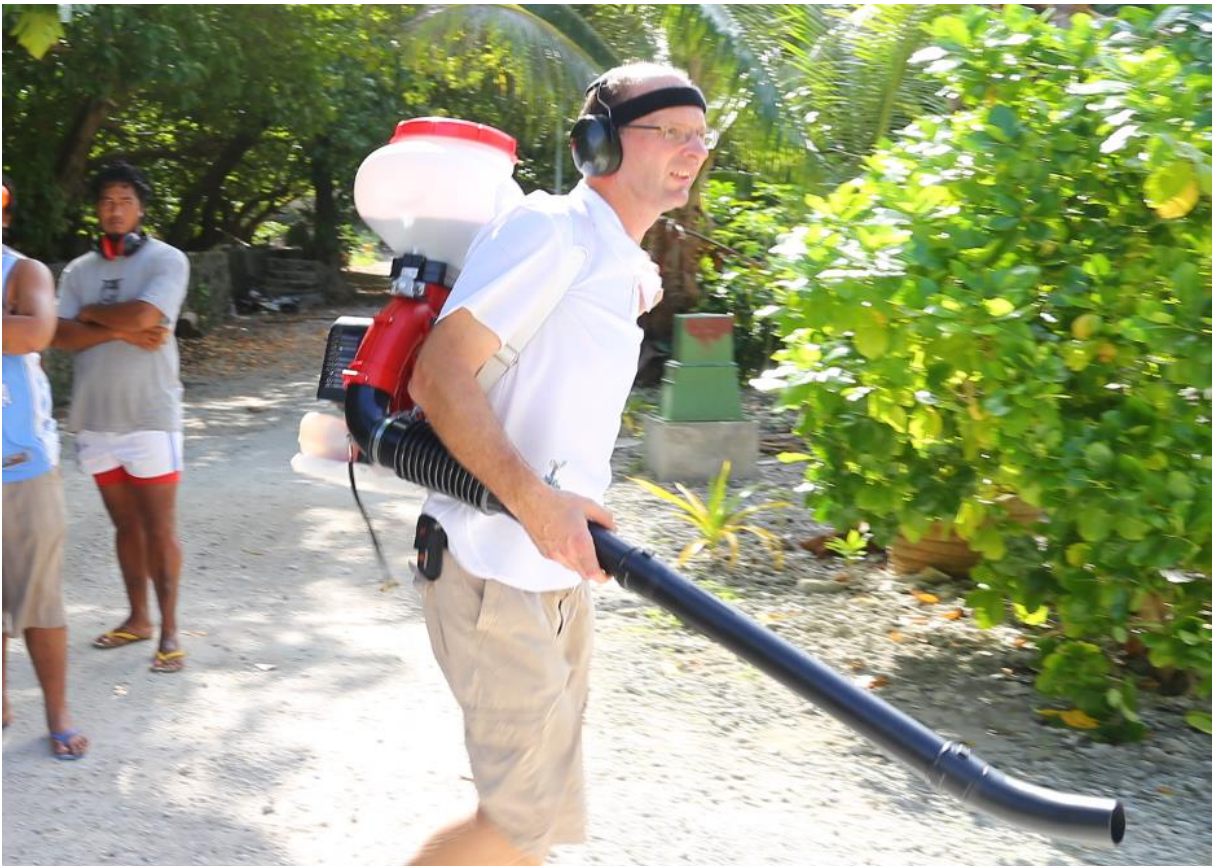
Figure 4: Back-pack mounted motorised blower used for distributing AntOff.
